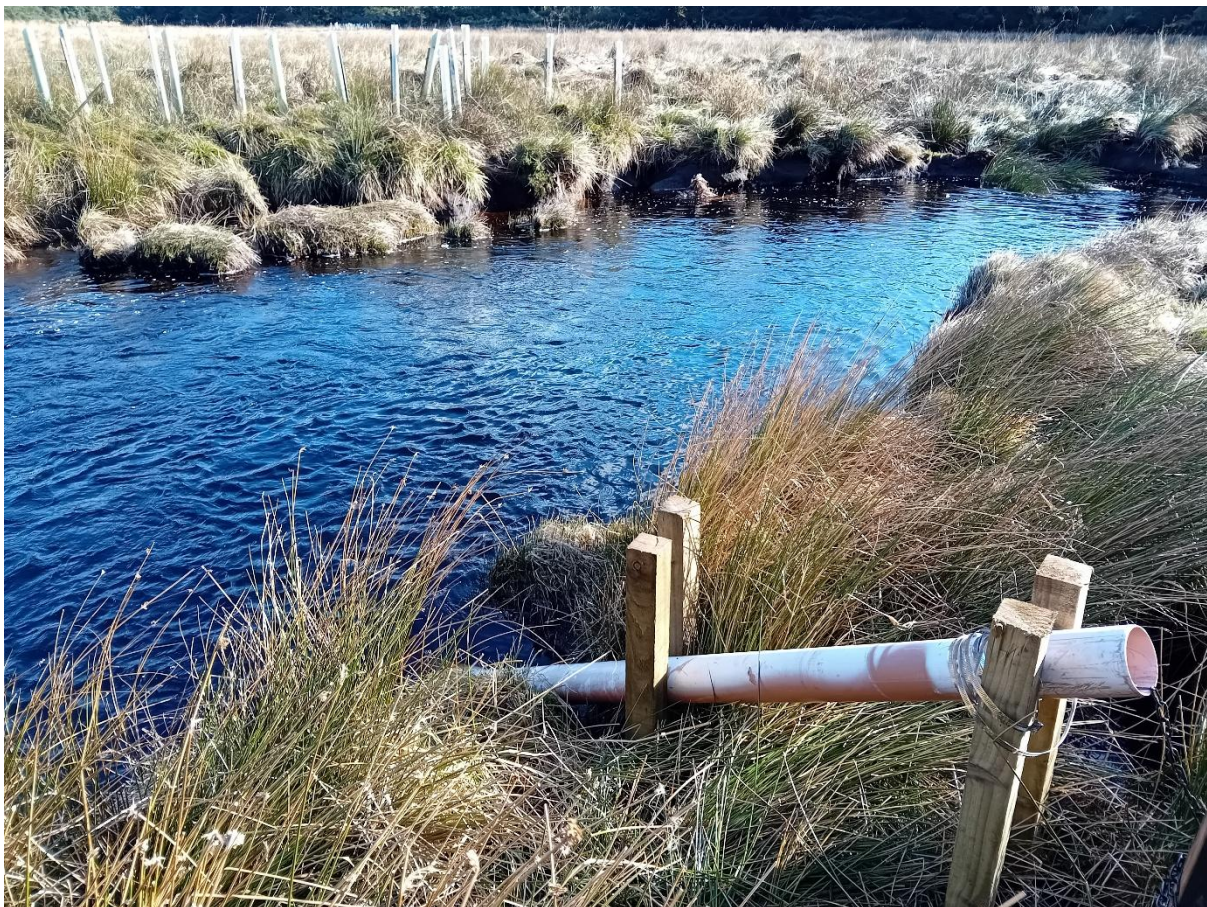
Picture 4: Example of GFT frame designed for the support of EXO1 Sondes
